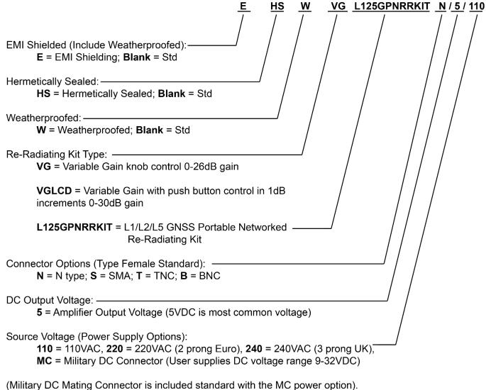
When no external power supply option (AC or DC) is selected, Output 1/J1 is Pass DC Standard. When external power supply option is selected, all outputs are DC blocked standard.
